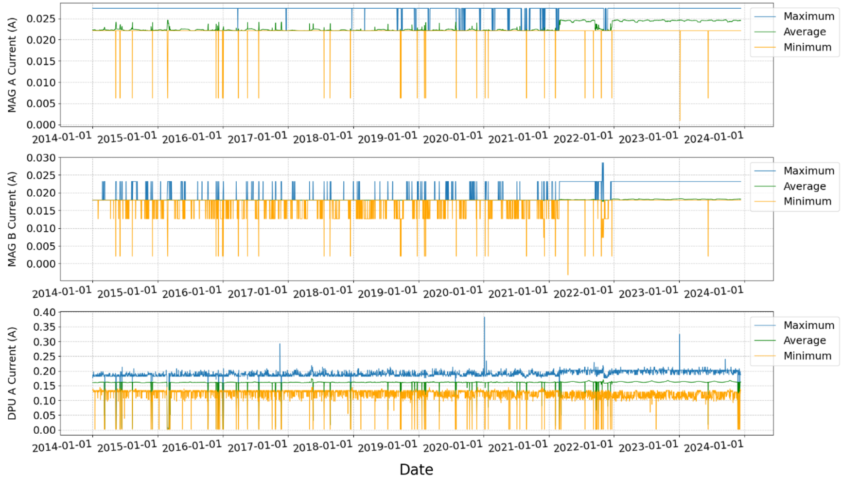
Figure 16: Top-to-bottom: Bus Magnetometer A current draw, Bus Magnetometer B current draw, and Star Tracker Digital Processing Unit (DPU) current draw for CASSIOPE/Swarm-E
