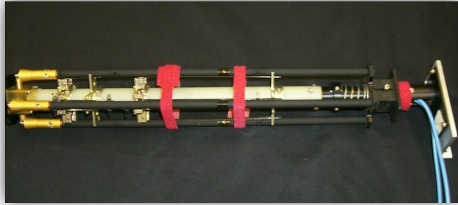
Figure 111: CERTO antenna in its stowed position
